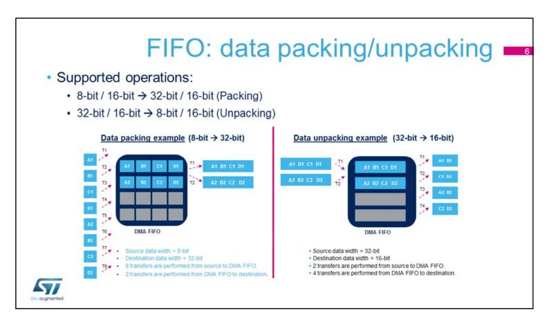
When FIFO mode is enabled (Direct mode disabled) the DMA controller manages the data format difference between source and destination (data packing and unpacking). thanks to its internal FIFO, the DMA stream can reduce software overhead and the number of transactions over the AHB Bus.
