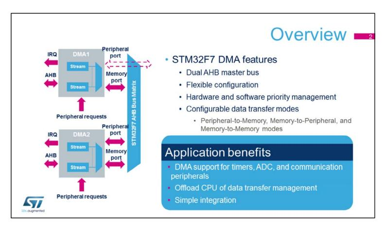
The STM32F7 has two Direct Memory Access controllers designed to efficiently support data transfers from peripherals and memories without any loading of the CPU. The DMA controllers are fully configurable and manage hardware and software priorities between streams as well as data transfer modes.
