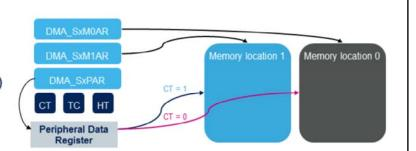
DMA controllers support Circular mode allowing to configure the number of data items to transfer once, and automatically restart the transfer after a Transfer Complete event. Double buffer mode is only available in Circular mode. It allows to switch automatically by hardware between two memory addresses each time a Transfer Complete event occurs. In double buffer mode, a status flag and control bit (CT) is available to monitor which destination is being used for data transfers
